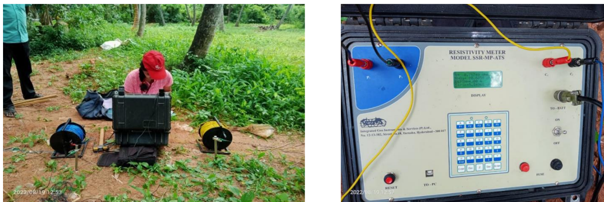
Fig. 3. Photograph shows VES Survey using SSR MP ATS Resistivity meter.
